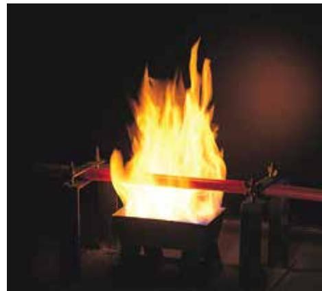
"Fire Retardant cables being tested by ISO: Accredited (750°C) at SQ Laboratory"
